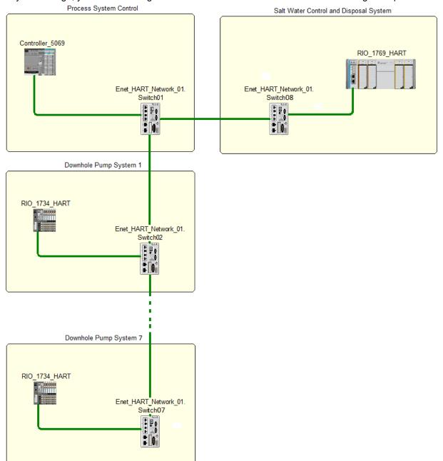
A process control system may have one system produced by one manufacturer, and multiple systems produced by another manufacturer, each using their own normal type of I/O to integrate into the Process Control System. In this illustration there are 3 Rockwell platforms integrated together—the 5069, 1734, and 1769 platforms.
