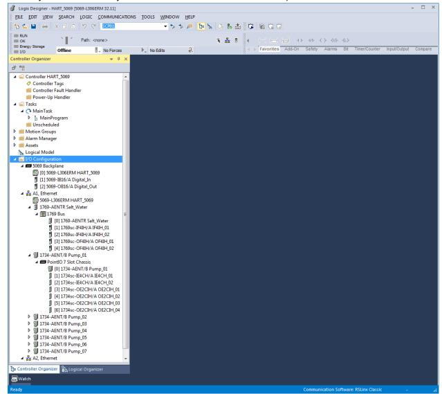
The 1734 HART I/O is a very popular choice because it automatically brings into the controller tags all four of the main HART variables for each enabled channel for a very low cost per module.
