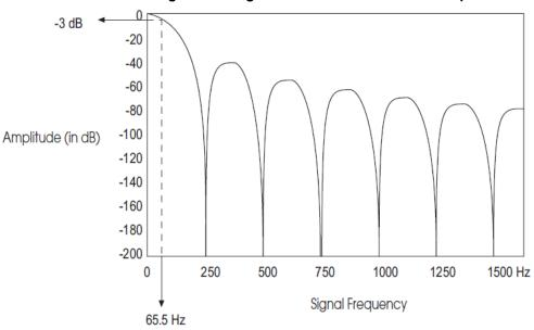
Figure 3-5. Signal Attenuation with 250 Hz Input Filter
