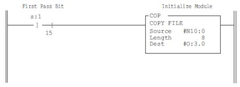
On power up, bit S:1/15 is set for the first program scan, and integer file N10 is sent to the NI8U channel configuration words.
