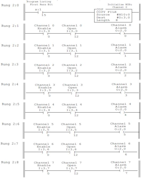
Figure 5-11. Data Table for Monitoring Channel Status Bits
