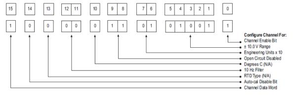
This example transfers configuration data and sets the channel enable bits of all eight channels with a single File Copy instruction.
