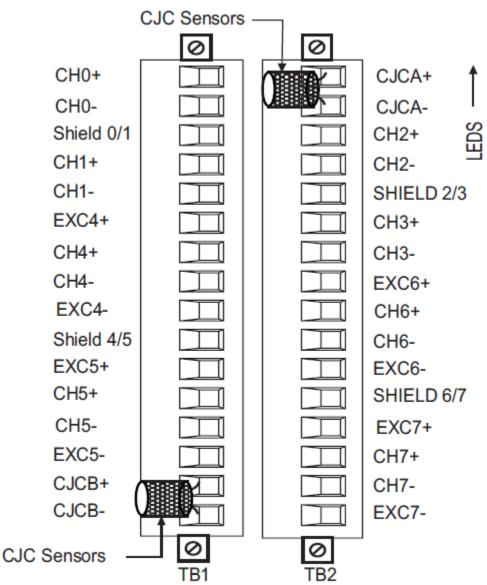
Figure 2-2. Terminal Block Diagram with CJC Sensors
