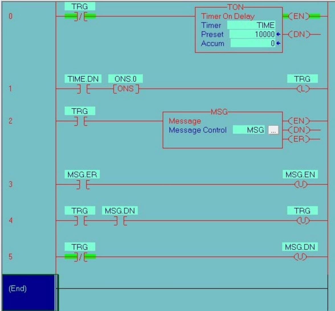
When the bit "TRG" is low the timer is enabled and runs for 10 seconds. When the timer is done the bit "TIME.DN" is set which latches the bit "TRG" enabling the message instruction. If the message instruction errors, it is reset and runs again. When the message instruction is successful it sets the bit "MSG.DN" which unlatches the "TRG" bit which in turn unlatches the "MSG.DN" bit and the process starts over again.
