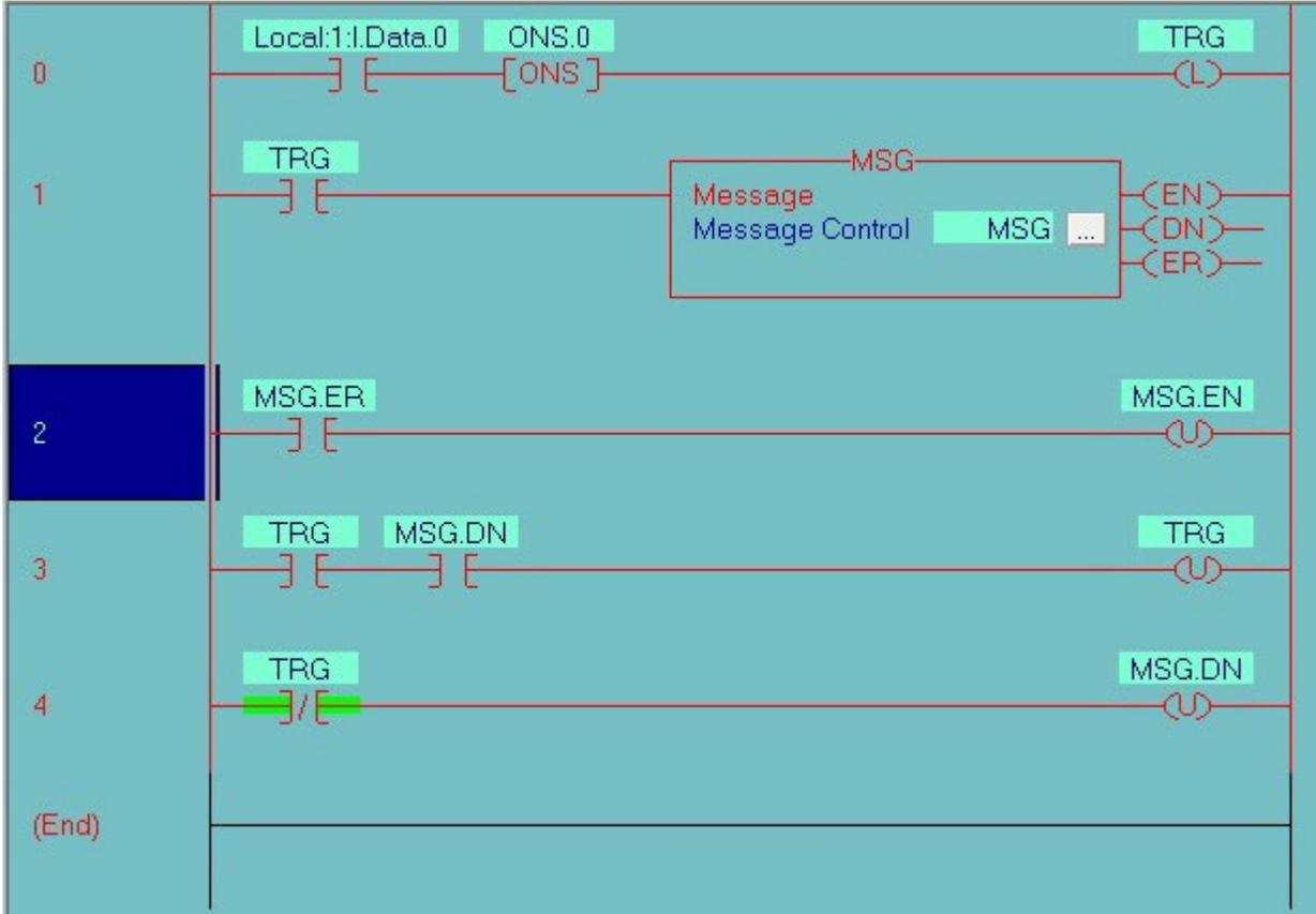
As with the time-based routine when the message instruction is successful the system is reset but will not execute the messaging until the discrete input opens then closes again. In both examples, in order to set up the Gateway to replace the NET-ENI, you need to know where the data is being read from and written to. One way to determine this is to look at the message instructions configuration (which is the same in both examples).
