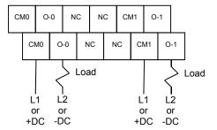
Note: In the diagram above, terminals with the same label are internally shorted together. Example, CM0 (Top Row) and CM0 (Bottom Row) are internally shorted together.
