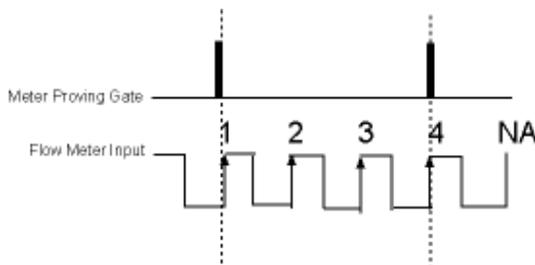
Given the above wave form, the module will begin counting the first positive going input pulse after the external enable input goes low. The module will accumulate 4 counts in the channel count register and stop when the external enable input goes high. The external enable line accommodates 5 Vdc, 12 Vdc and 24 Vdc signals and is pulled low internally.
