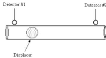
The Meter Proving Inputs are designed for use with typical meter proving applications. These inputs differ from the hardware inhibit/trigger inputs in the way they start and stop the counter.
