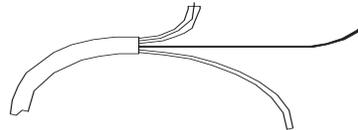
5. At the other end of the cable, cut the drain wire and foil shield back to the cable and apply shrink wrap.
