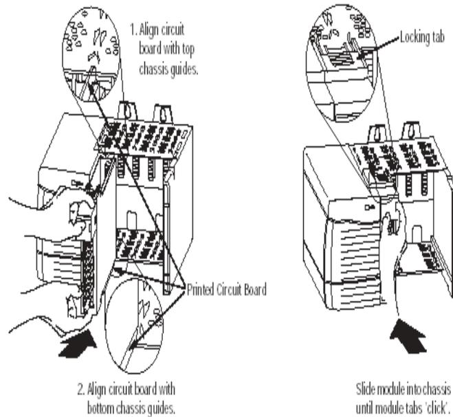
2. Slide your module into the chassis until both top and bottom retaining clips are secure. Apply firm even pressure on your module to attach it to its backplane connector. Never force your module into the slot.
