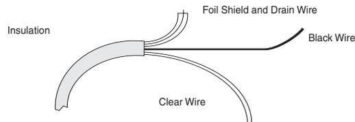
6. Connect the wires to the terminal block and field device as shown in the following figures and table. The recommended maximum torque is 4.5 in-lb (0.565 Nm) for all terminal screws.
