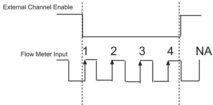
Given the above wave form, the module will begin counting the first positive going input pulse after the external enable input goes low. The module will accumulate 4 counts in the channel count register and stop when the external enable input goes high.
