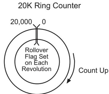
The above figure illustrates counting in a clockwise direction.
