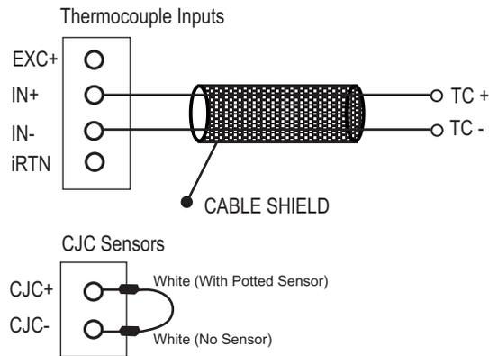
For cold junction compensation be sure the two supplied thermistors are connected. One should be connected between CJC0-IN+ and CJC0-IN- and the other should be connected between CJC1-IN+ and CJC1-IN-. Also be sure configuration tag “.CJDisable” is set to zero to perform cold junction compensation for thermocouple inputs
