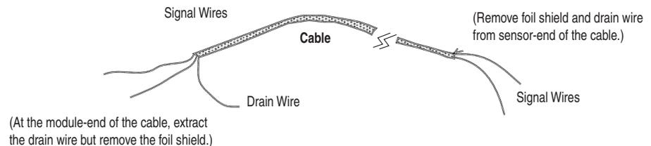
1. At each end of the cable, strip some casing to expose individual wires.
