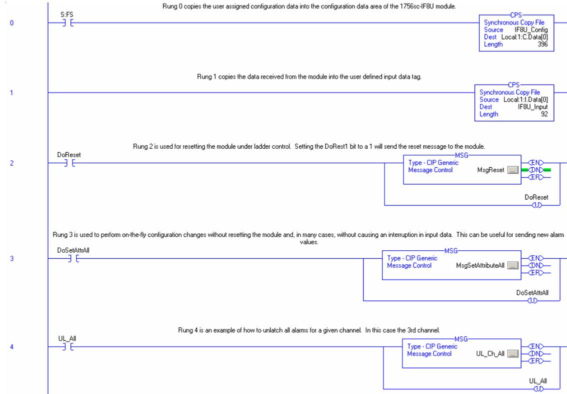
Rung 0 - This rung copies the configuration data (IF8u\_Config) into the module's configuration image memory. This rung is required.
